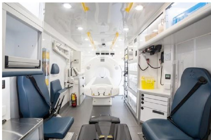
Figure 7: University of Tennessee Memphis Mobile Stroke Unit equipped with 16-slice Siemens Somatom Scope® scanner and head/neck CTA autoinjection system; with permission from University of Tennessee Health Science Center at Memphis, Mobile Stroke Unit
